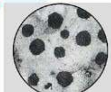
Microphotograph for ductile cast iron
