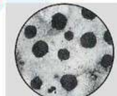
Microphotograph for ductile cast iron
