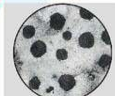
Microphotograph for ductile cast iron
