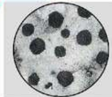
Microphotograph for ductile cast iron
