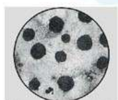
Microphotograph for ductile cast iron
