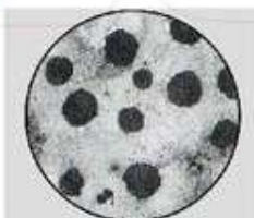
Material: ductile iron FCD-60.
