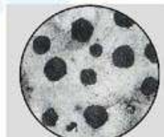
Microphotograph for ductile cast iron
