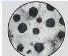
Microphotograph for ductile cast iron
