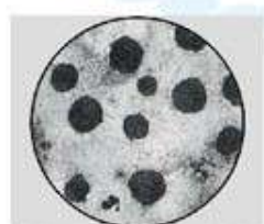
Microphotograph for ductile cast iron
