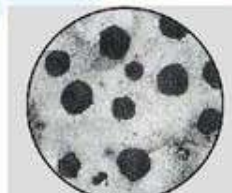
Microphotograph for ductile cast iron
