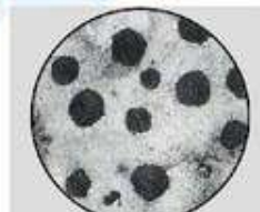
Microphotograph for ductile cast iron
