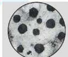
Microphotograph for ductile cast iron
