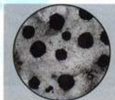
Microphotograph for ductile cast iron
