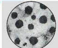
Microphotograph for ductile cast iron
