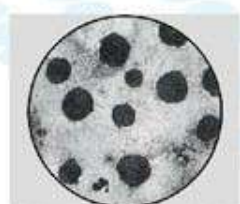
Microphotograph for ductile cast iron
