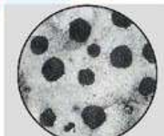
Microphotograph for ductile cast iron
