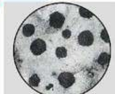
Microphotograph for ductile cast iron
