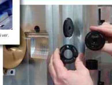
PinLock locating system installed in a tombstone
