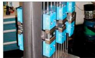
Solution: Two-sided tombstone with six MoveLock clamping stations handle wide range of part sizes.
