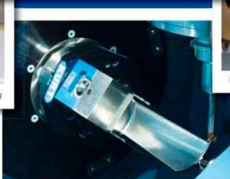
MaxLock 5 axis vise used for turbine blade machining
