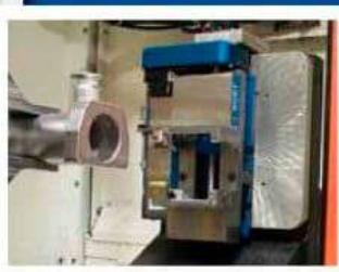
Air powered vise used in a robotic cell
